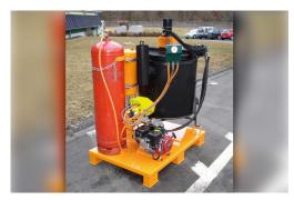
Equipment for melting and processing thermoplastic road marking materials, bituminous joint sealing, rail sealing and railway grouting materials
