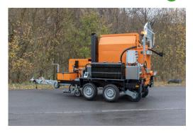
Equipment for melting and processing bituminous joint and rail sealing material
