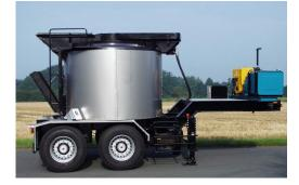
Special equipment for transporting mastic asphalt and mastic.
