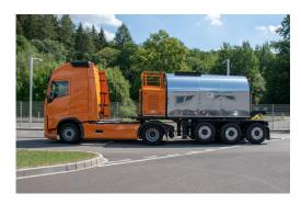
Special equipment for transporting mastic asphalt and mastic.
