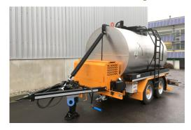
For the transport of primer, bitumen emulsions and polymer-modified binding material
