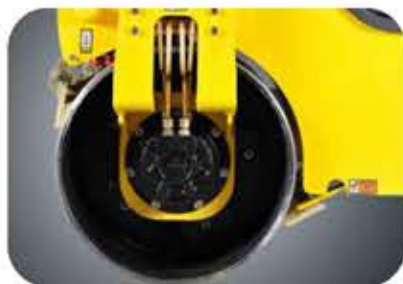
Big drum diameter makes compaction easier even on soft tricky asphalt mixes and thick drum shells for longer life-span
