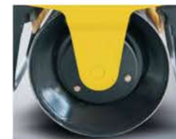
Thick drum shells for longer drum life.
